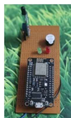
(c) IoT based Fire Alarm
