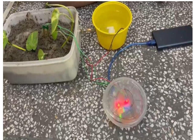
Fig 10. Pump On when Dry (Relay NO Activated)
