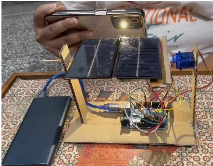
Fig 8. Solar Panel Moving Towards High Intensity Light
