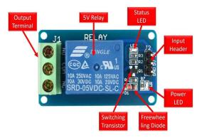
When activated, the electromagnet pulls to either open or close an electrical circuit.
