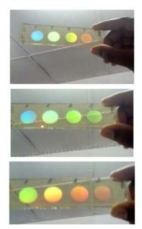
Fig. 3. Transmission Holographic Lens Recorded by Three Visible Laser Wavelengths.
