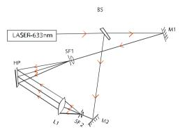
Fig. 1. Schematic of holographic lens recording
