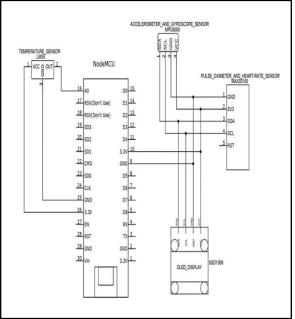
Figure 2: Circuit Diagram of the wearable device
