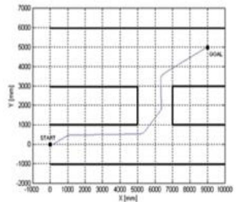
Figure 1: The linear path the Robot travels in tangential approach
