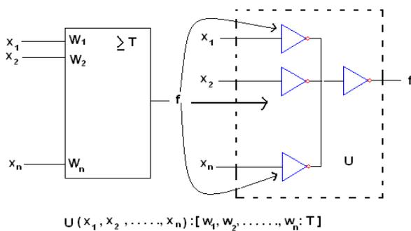
Figure2: Nonstandard symbol of Threshold gate and threshold gate basic structure using output wired ganged CMOS .
