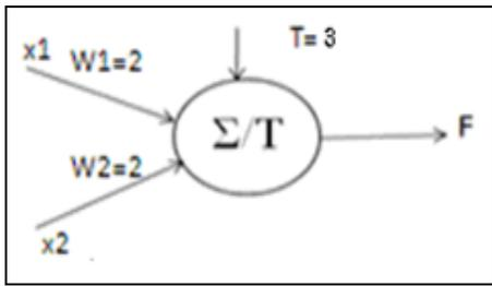
Figure 1: Design of Threshold logic based AND gate
