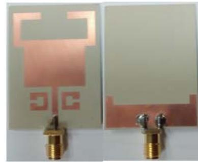
Fig. 7. Fabricated prototype of the proposed antenna.
