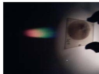
Fig. 4. Spectrum splitting of Holographic Solar Concentrator
