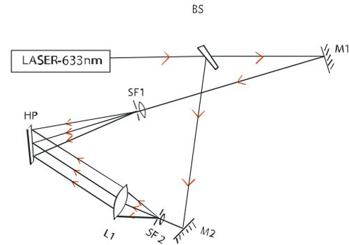
Fig. 1. Schematic of holographic lens recording
