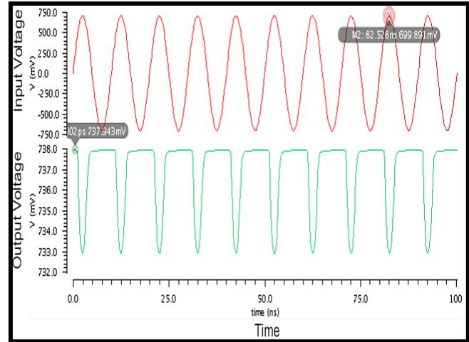
**Fig.6.** Output of Proposed 2-Stage OTA
