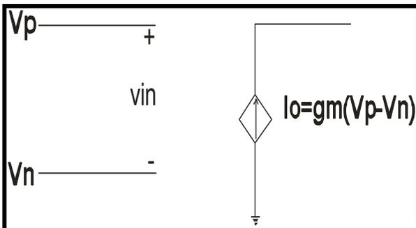
Fig 2: Equivalent circuit of OTA
