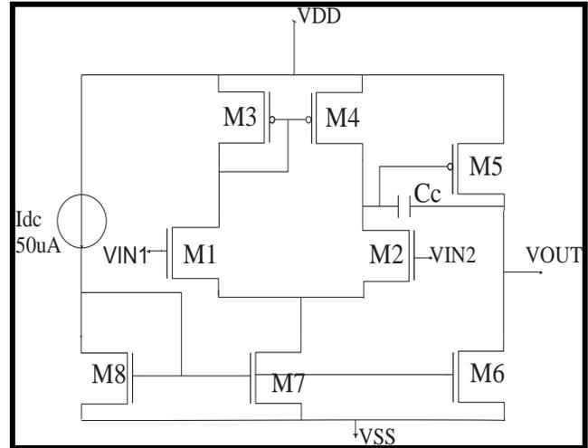
Fig.3. Conventional diagram of 2-Stage OTA
