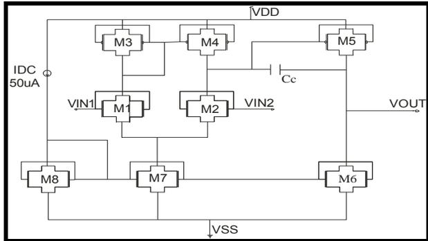
**Fig.5.**Proposed diagram of Two-stage OTA by FinFET Technique
