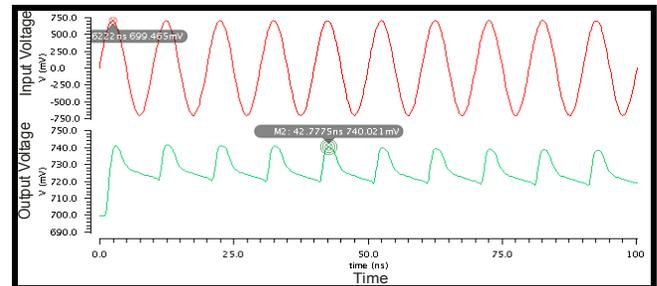
Fig.4. Output of Conventional 2-Stage OTA
