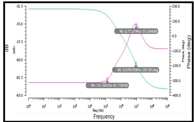
**Fig.9.** Phase Margin and Gain Margin
