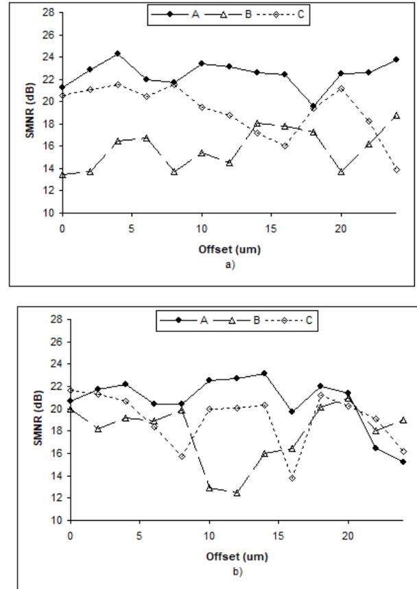
Fig. 3: SMNR results for configurations A, B, C with a) 220 m and b) 300 m MMF length.
