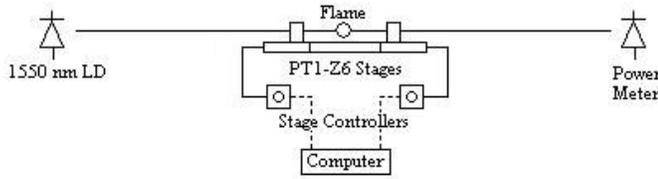
Fig. 1: Taper Fabrication Setup
