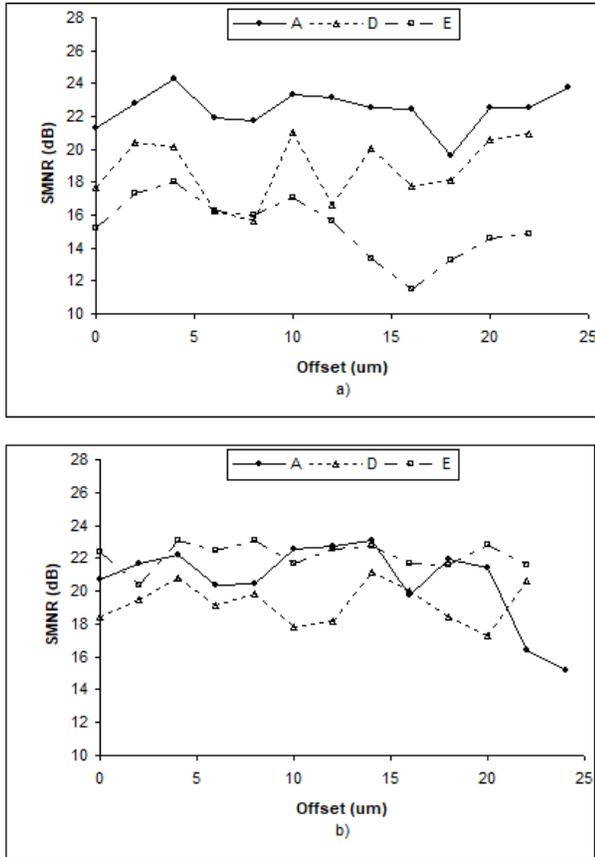
Fig. 4: SMNR results for configuration A, D, E with a) 220 m and b) 300 m MMF length.
